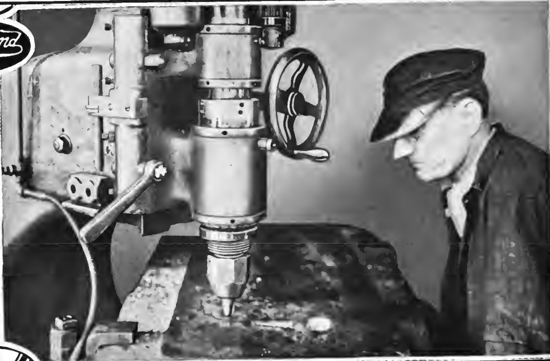
A—Depicting a Vertical Routing Machine Routing Out for a Breaking-down Die to Be Used in Drop-forging, Special Steel I-Section Front Axles
